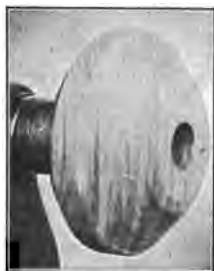
Fig. 209. Base Roughed Out.
